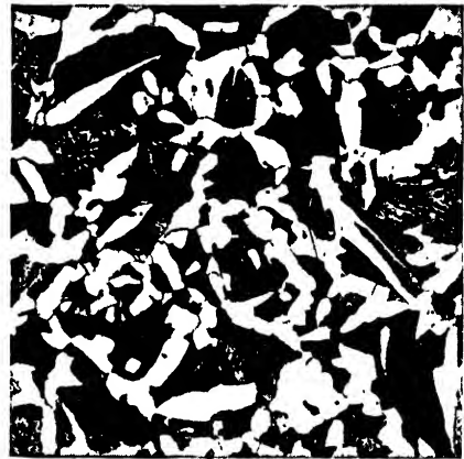
FIGURE 468. Metallographic structure of a cast steel containing about 0.40% carbon. Etched with nital.
